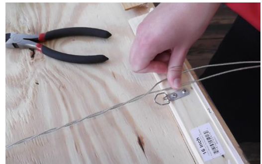
Figure 18. Wire is twisted too tightly
