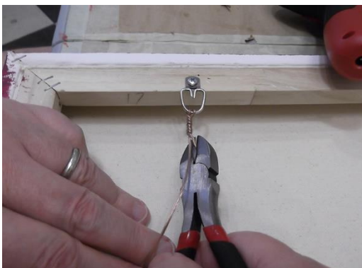
Figure 7. Cutting off the excess
