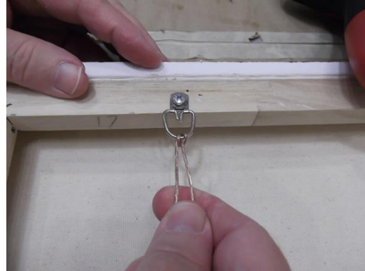
Figure 4. Pulling the end tight to form the lock
