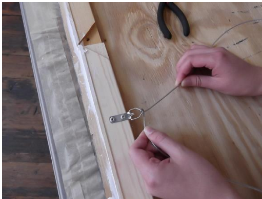
Figure 15. Starting the lock stitch in the middle of the wire on the left D-ring
