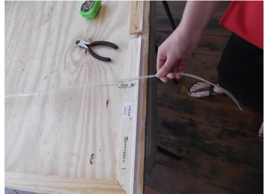
Figure 14. About a foot of extra wire is left on each end past the right D-ring
