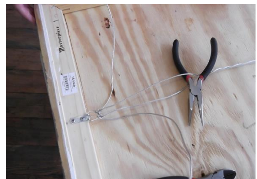
Figure 24. Holding the wires apart with plier weight
