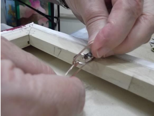
Figure 3. Pulling the end up tight against the main wire and running it back through the D-ring
